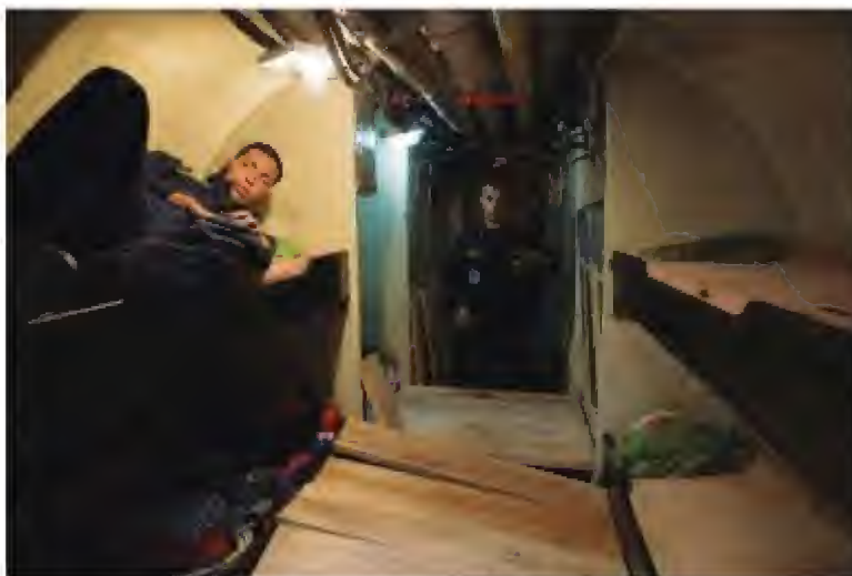
Made with three-centimeter-thick fiberglass, the submarine has a 346-horse power engine, space for a crew of four, a range of about 900 miles and the capacity to transport 8 tons of cocaine.
